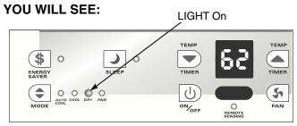
**Note:** Use this mode when the room is already cool below  $65^{\circ}F(18^{\circ}C)$  but the room is slightly humid.
